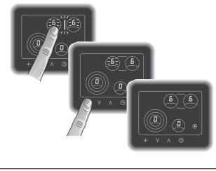
Both rear cooking zones convert together with an additional zone, to create an oval cooking zone especially suitable for roasters. In the options menu it is possible to choose the oval cooking zone as the standard cooking zone.
